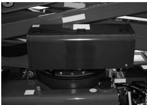
Fig. 120 Aerial part distributor protection
