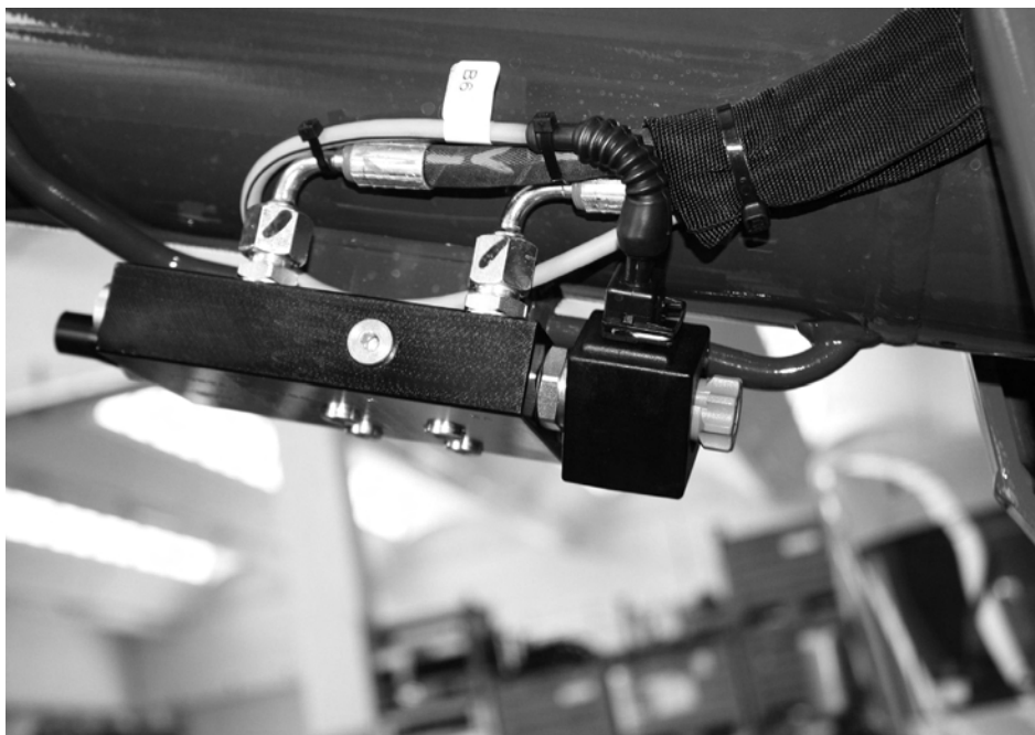
Fig. 66 Solenoid valves for emergency descent
