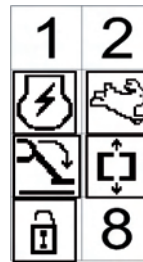
Fig. 127 Emergency BY-PASS activated
